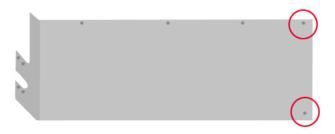
b. Lift the side panel and slide in the 2 rear wing nuts (do not tighten them). Insert the tool though the middle hole of the panel to align with the middle the preloaded Slide-in Thick Nut. Fasten loosely with a Stainless Steel screw.
