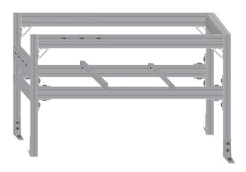
11. Attach the sides to the frame, using the 18 stainless steel screws
